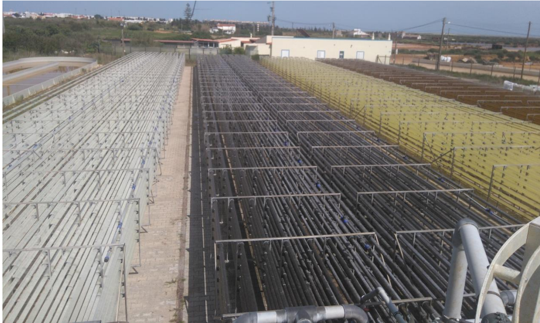
Figure 3.4 Four tubular systems of photobioreactors. Microalgal culture is pumped through the horizontal tube. The photobioreactor at the left is without culture, the others contain culture of different species and densities.
