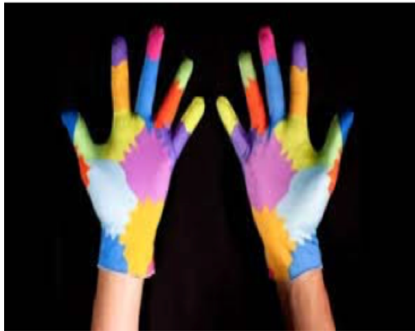
Figure 2-2: Color Marker based hand Gesture Recognition [2]
