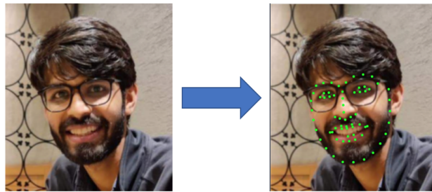
Fig. 4. Sixty-Eight facial landmarks plotted on a sample test-image 2.
