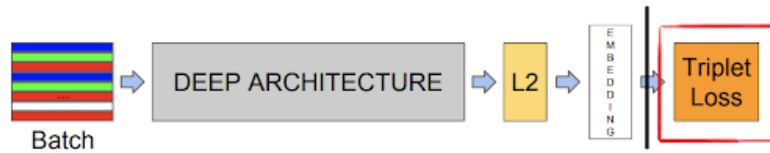
Fig. 11. Triplet loss block diagram of FaceNet by Schroff et al. [1]
