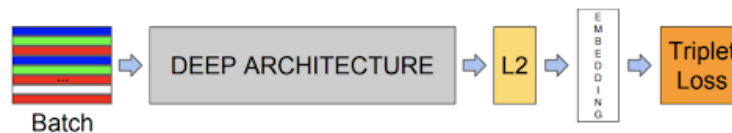
Fig. 10. Block diagram of FaceNet by Schroff et al. [1]
