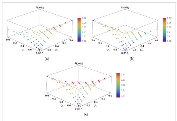
**Figure 2.** The fidelity of the target state versus  $\mathcal{O}_z$  and  $\mathcal{O}_x$  for three different noise strength ratios. (a)  $\eta_x=0.125$  kHz and  $\eta_z=\eta_x/2$ . (b)  $\eta_z=0.125$  kHz and  $\eta_z=\eta_z/2$ . (c)  $\eta_z=\eta_x=0.125$  kHz. In all the plots  $\Delta_0=10$  kHz and  $t_f=0.5$  ms. Maximal fidelity is always found for minimal  $\bar{\mathcal{O}}$ .
