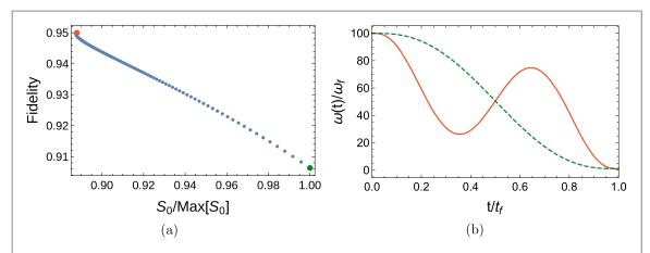
**Figure 3.** (a) Fidelity versus the normalized  $S_0$ . Each point in the figure corresponds to a different control. (b) The control frequency  $\omega$  (t) as a function of t for the green (dashed) and red (solid) points. Parameter values:  $\nu_0 = \omega_0/(2\pi) = 15.92$  MHz,  $\omega_f = \omega_0/100$ ,  $\eta = 10$  Hz Å $^{-2}$ , and  $t_f = 100$   $\mu$ s. The initial coherent state is given by  $\alpha = 1 + i$  and the final state by g = 50.5  $\mu$ s.
