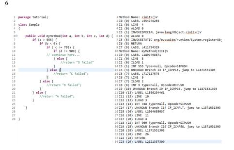
Fig. 2: A simple Java class. Source code is on the left and bytecode is on the right.
