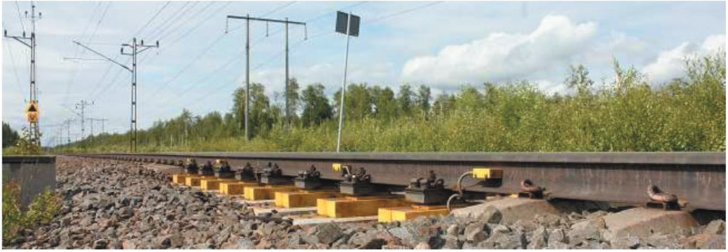
Figure 1. Wheel impact load detector [14] at Sunderbyn. Photo by Matthias Asplund, Swedish Transport Administration.
