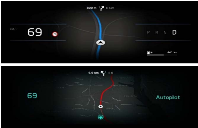
Fig. 2. Top: The HMI view in manual mode. Bottom: The HMI view in automated mode.
