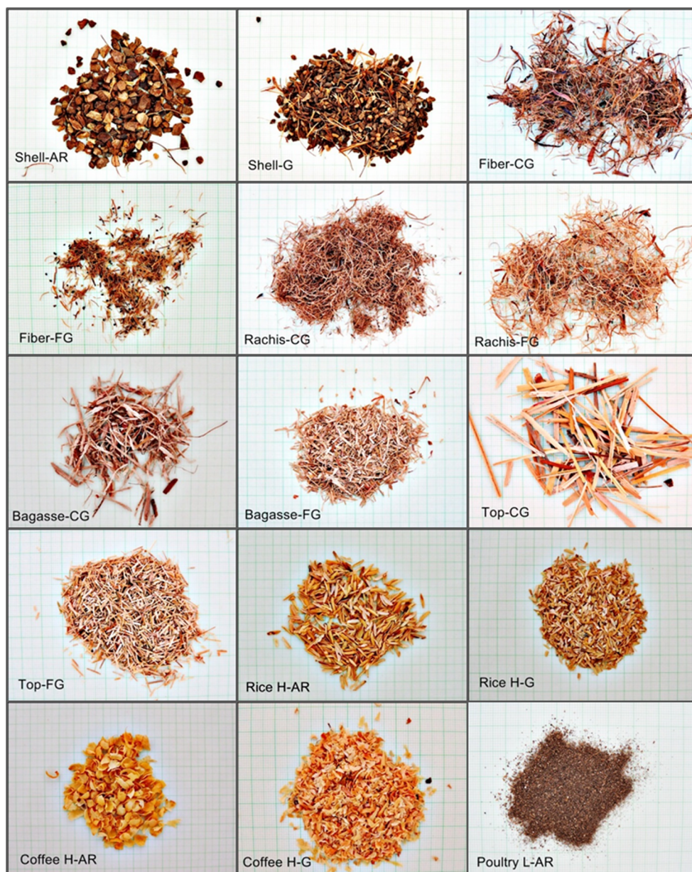
Fig. 1 Pictures of the biomass samples after the conditioning processes: oil palm shell as received (Shell-AR), oil palm shell ground (Shell-G), oil palm fiber coarsely ground (Fiber-CG), oil palm fiber finely ground (Fiber-FG), oil palm rachis coarsely ground (Rachis-CG), oil palm rachis finely ground (Rachis-FG), sugarcane bagasse coarsely ground (Bagasse-CG), sugarcane bagasse finely ground (Bagasse-FG), sugarcane top coarsely ground (Top-CG), sugarcane top finely ground (Top-FG), rice husk as received (Rice H-AR), rice husk ground (Rice H-G), coffee husk as received (Coffee H-AR), coffee husk ground (Coffee H-G), and poultry litter as received (Poultry L-AR)
