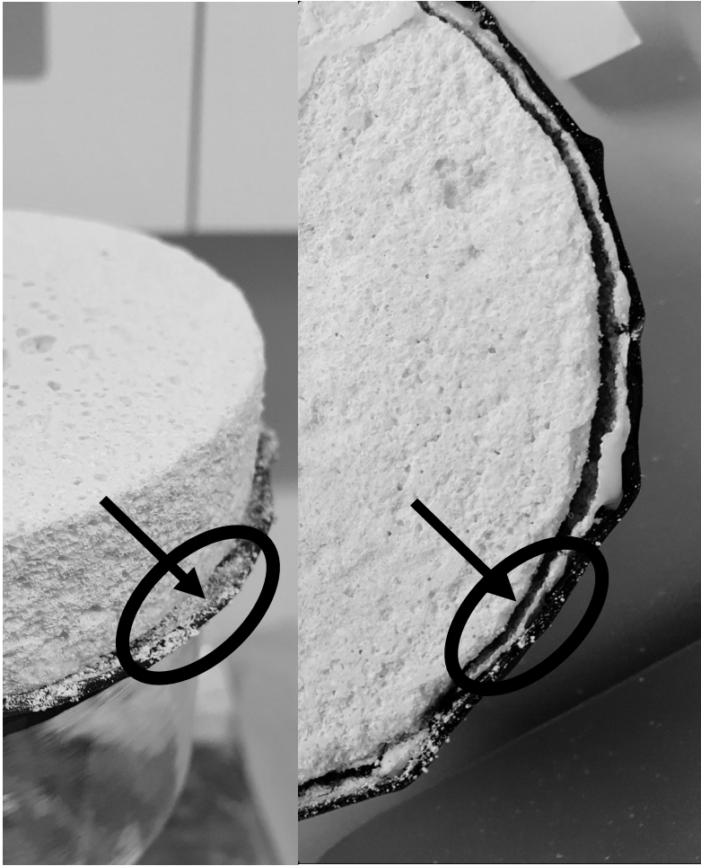
Figure 10. Photos showing sealing attempts of AP samples for cup method test. Left: Detaching of the butyl tape from the surface of the AP sample. Right: Wax detaching from the surface of the AP sample.
