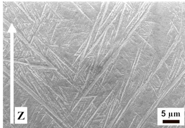
Figure 15: Scanning electron micrograph of Ti-6Al-4V built by L-PBF along the building direction.
