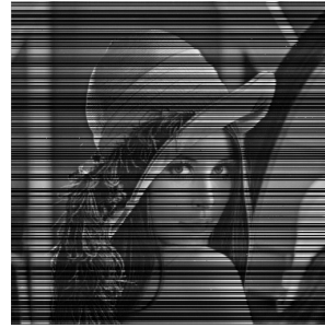
(c) Decoded image without information about source coding, BER = 0.2673
