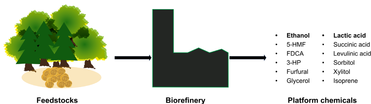
Figure 1: The concept of a biorefinery for the biochemical conversion of lignocellulose into potential platform chemicals. The listed platform chemicals were identified by the US Department of Energy (Bozell & Petersen, 2010). Ethanol and lactic acid (highlighted in bold) were selected as products in my thesis to demonstrate the application of biorefineries for platform chemical production and to discuss the development of process designs to improve process performance. 5-HMF, 5-Hydroxymethylfurfural; FDCA, 2,5-Furandicarboxylic acid; 3-HP, 3-Hydroxypropionic acid.
