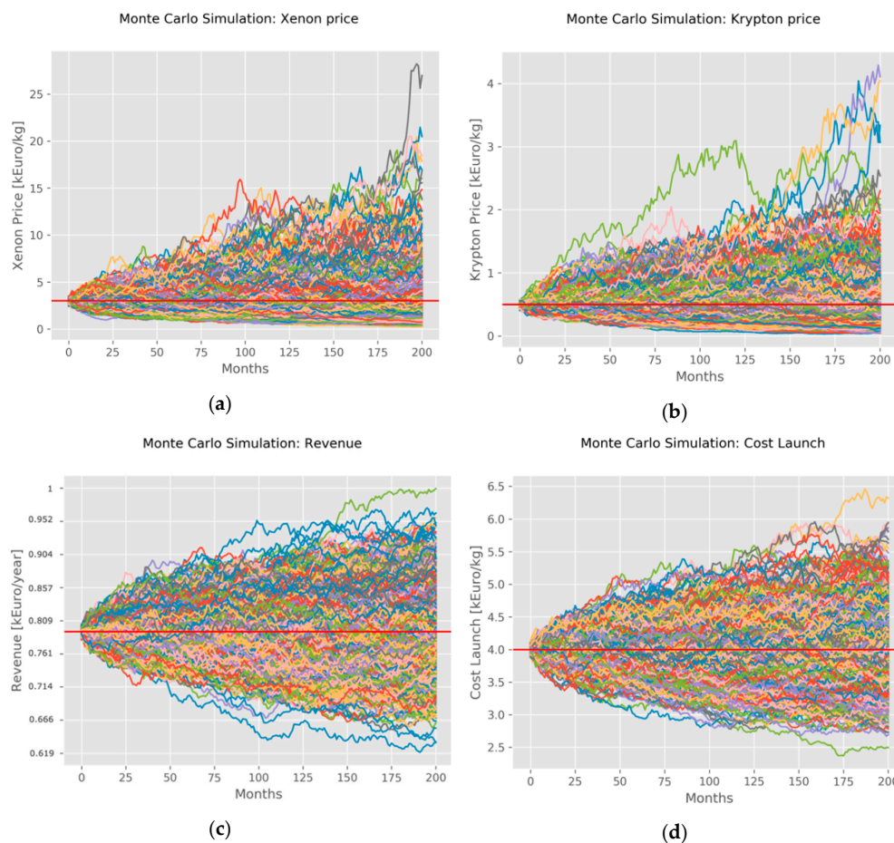
Figure 7. 1000 scenario variations of market input data based on the Wiener stochastic model: (a) xenon price; (b) krypton price; (c) revenue per year; (d) cost launch per kg. The data regarding the revenue per year (c) are normalized to preserve company sensitive information. Each color line represents a single scenario (1000 scenario variations in total).
