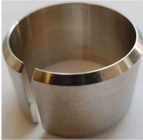
Figure 18: Picture of a finished sample ring, used for probe exposures in the field-studies.
