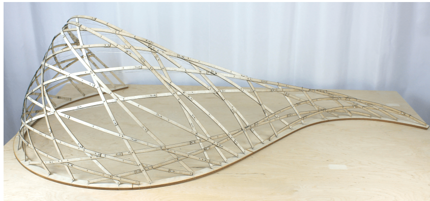
Figure 4: 1:10 scale model of the main shell of the pavilion where both size and stiffness properties were scaled.
