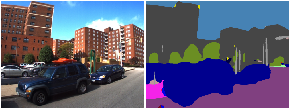
Figure 2.6: An image from the CMU Visual Localization dataset and its corresponding semantic segmentation.
