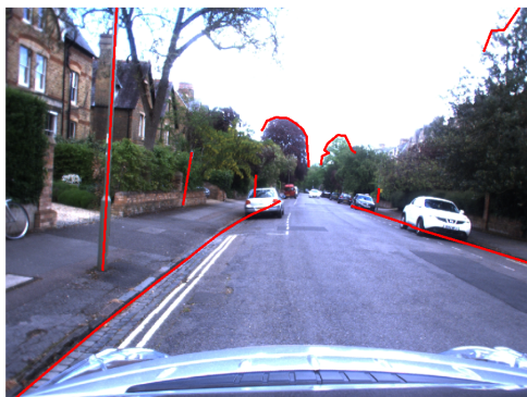
Figure 3.1: Illustration of the method in Paper I. Any given pose may be evaluated by how well the semantically labelled structure projects down into the given pose. Only the semantic 3D curves are shown (poles, road edge, vegetation-sky contour). 3D points (not shown) were used as well.
