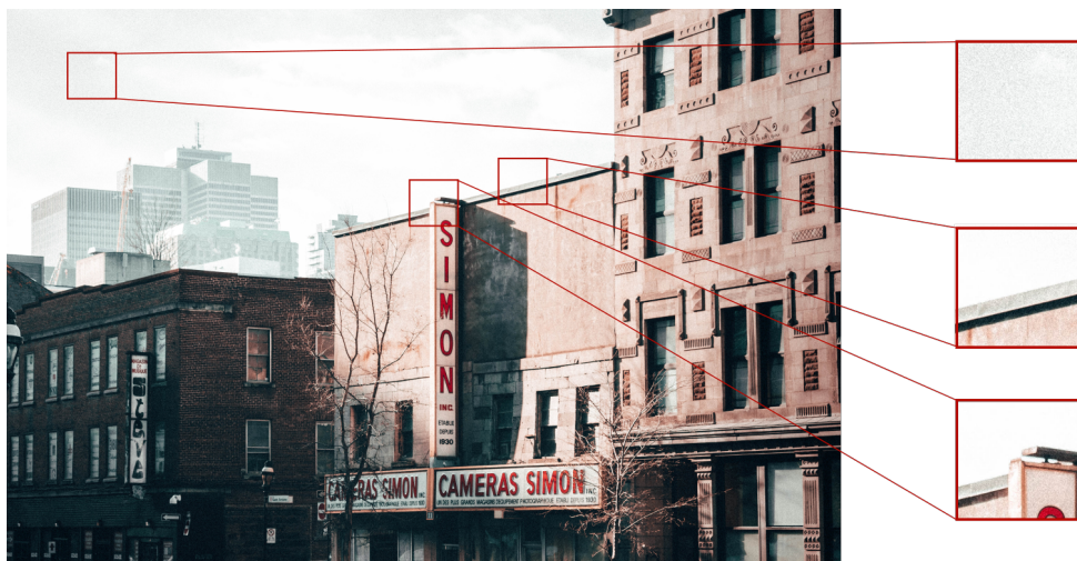
Figure 2.1: Three example image patches from an image. A feature detector should trigger on corner-like points we believe we could re-identify in a different image. Do you think you could find and correctly match the three extracted patches in a different image of the same scene?
