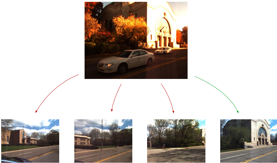
Figure 2.5: Visual place recognition formulates the localization problem as an image retrieval problem. Given a query image and a set of database images, find the database image most similar to the query image (according to some metric).
