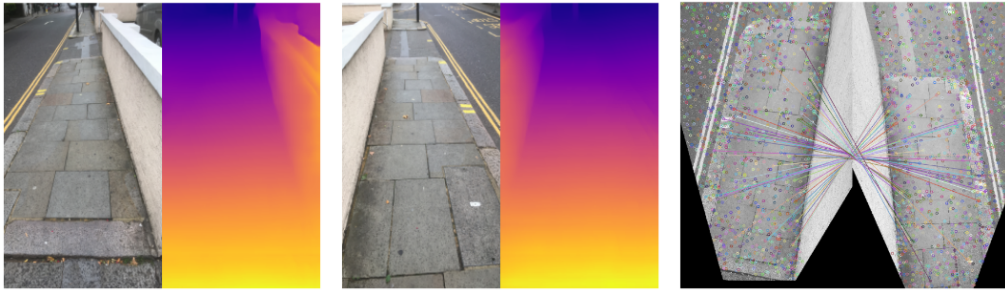
Figure 3.3: When matching features between images taken from very dissimilar viewpoints (such as the left and middle image here), we can use pixelwise monocular depth predictions (shown next to the images) to render a top-down view of the images and match features in these top-down views (right).
