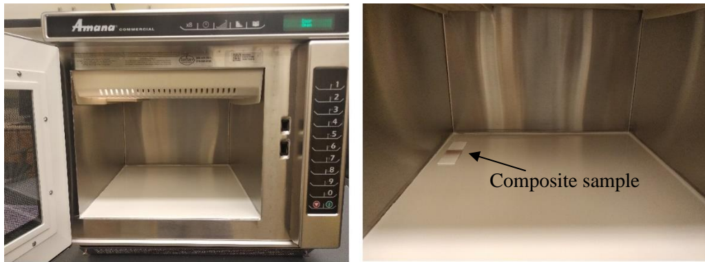
Fig. 20. A picture of the Amana microwave oven used for this study. A sample is shown in the oven chamber close to the wall.
