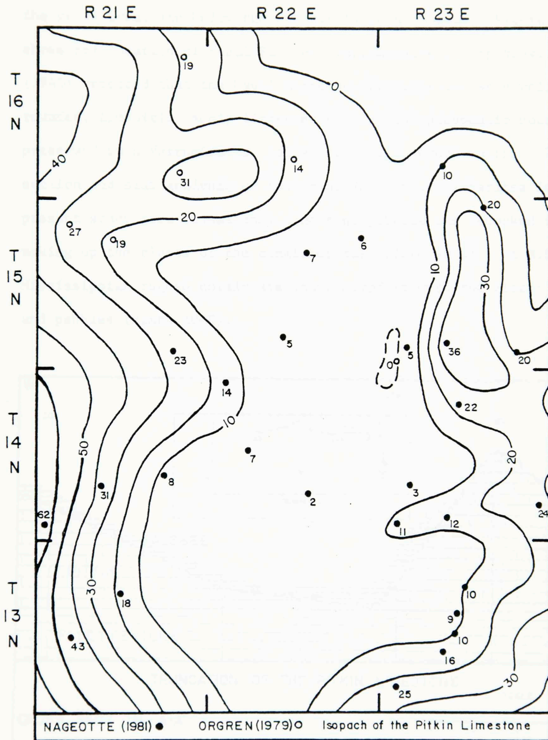
Figure 16. Isopachous map of the Pitkin Limestone in portions of Cherokee, Muskogee, and Sequoyah Counties in northeastern Oklahoma. A 10 foot contour interval is used. Solid circles are from sections measured in this study, open circles are from Orgren (1979).
