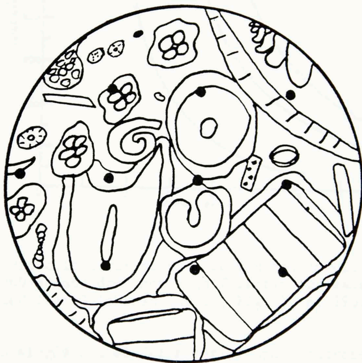
Figure 4. A grid of points is used to count constituent grains in thin sections by the Glagalev-Chase method. The result of this method is an estimate of the volume percent of the constituent grains (modified from Galehouse, 1971).
