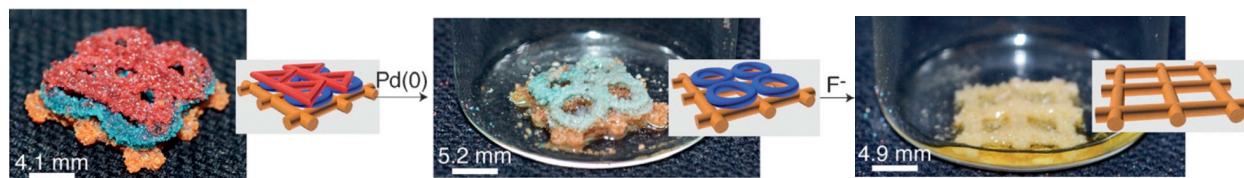
Figure 9. Visual ion sensors based on PPAb (red triangles, blue circles, and yellow grids are Pd(0), fluoride ion, and non-responsive PPAs respectively). Adapted with permission from reference 75 . Copyright 2015, John Wiley and Sons.
