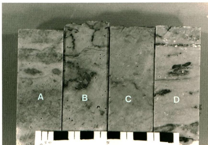
PLATE 24. Typical Transition Zone microstylolite swarm. Scale in cm.
