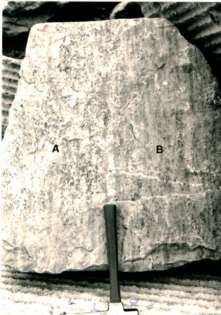
PLATE 14. A slab of Amabel Dolostone cut parallel to the bedding,
