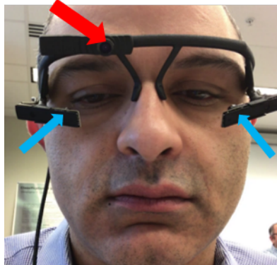
Figure 5: Pupil Pro Head Mounted Eye Tracker. World tracker camera (red) and IR eye tracking cameras (blue) are used to provide gaze estimates and visual overlay using the Pupil Capture application.
