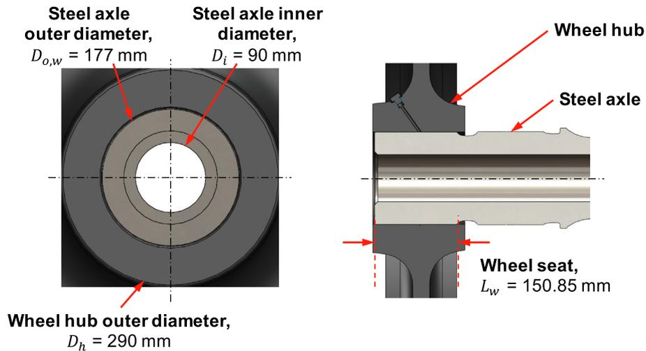
Fig. 8. Wheel hub press-fit onto hollow steel axle.
