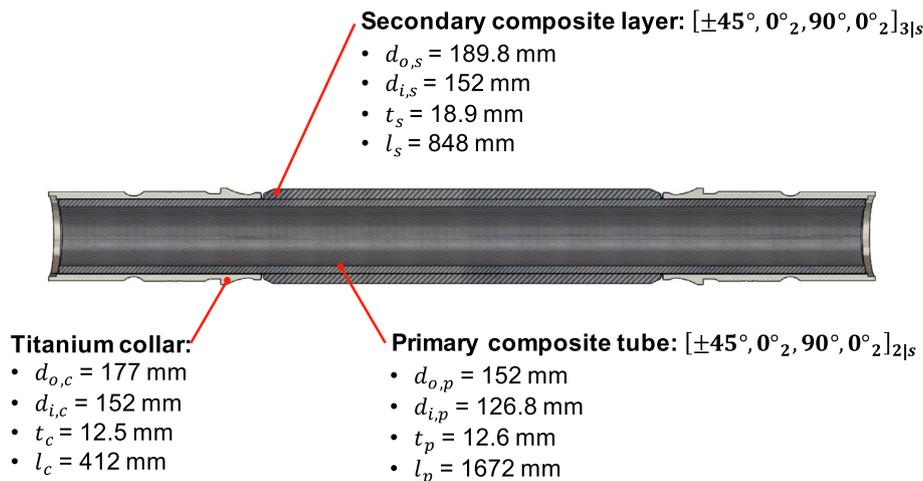
Fig. 13. Recommended solution for the full-length pre-manufactured tube axle design concept. Where, *d*, refers to the diameter of the tube, *t*, refers to the thickness of the section and *l*, refers to the length of the section.
