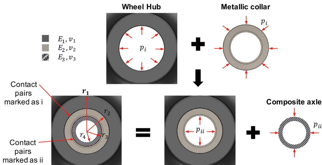
Fig. 10. Superposition principle of tri-layer thick-walled cylinders assembled from outside to inside. Here,  $E$ , is the Young’s modulus and  $\nu$ , is the Poisson’s ratio. Subscript 1, refers to the wheel hub, subscript 2, refers to the metallic collar and subscript 3, refers to the primary composite tube.
