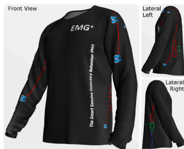
Figure 16. A revised version of the EMG+ (accelerometer not shown) to improve its suitability for field use. The smart shirt uses only the three most relevant EMG channels presented in Paper I, including one reference electrode. Abbreviations: Electromyography plus Accelerometer (EMG+), Electromyography (EMG).
