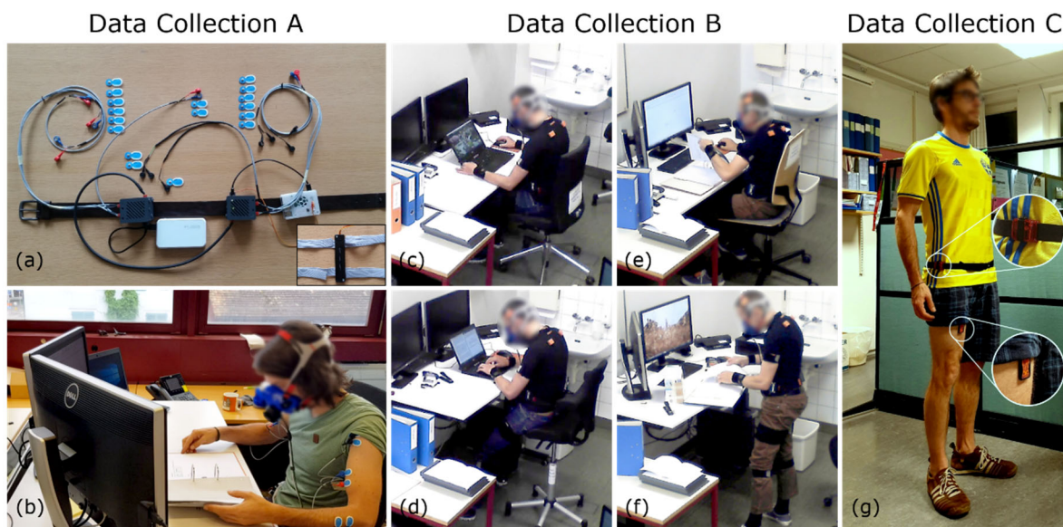
Figure 5. Illustrative pictures for each data collection. a) the EMG+; b) Participant performing the Deskwork task on Conventional Chair; c) Mouse task on Conventional Chair; d) Typing task on Saddle Chair; e) Deskwork task on Active Chair; f) Sorting task at Standing Desk; g) sensor placement in data collection C. Task and workplace explanations are given in Table 3 (p. 24). Picture a, b and g previously published under CC BY license in MDPI journals. Abbreviation: Electromyography plus Accelerometer (EMG+).
