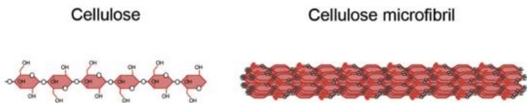
Figure 1.1. Chemical structure of cellulose and cellulose microfibrils.
