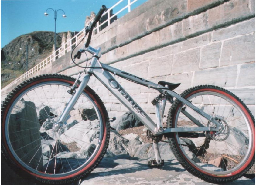
Figure 14: Stock bikes through the ages. From top down: a) Azonic DS-1 16 inch duel slalom frame: it has no bashguard, but instead an unused 32tooth chainring that has had the teeth ground off. Conventional saddle, 8 gears and suspension forks. b) Orange Zero: One of the first breed of specific trials frames. Features high bottom bracket, low mini seat, FSA branded cranks and bashguard. c) Zoo piranha 09 frame: modern trials frame, no seat option for low weight and maximum clearance, single gear with small bashguard. Photo credit from top: Tom, author, Laurent.
