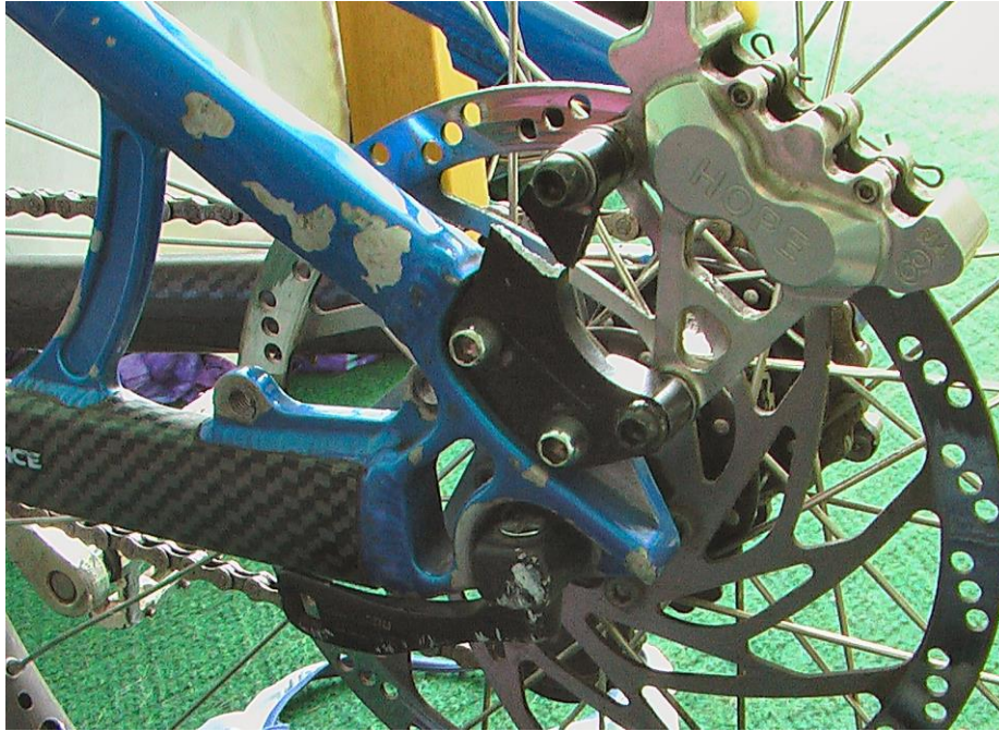
Figure 27: Broken disk mount, a serious but not uncommon trials related failure. This design attempts to cope with this by using a replaceable mount, designed to break in preference to the bike frame itself.
