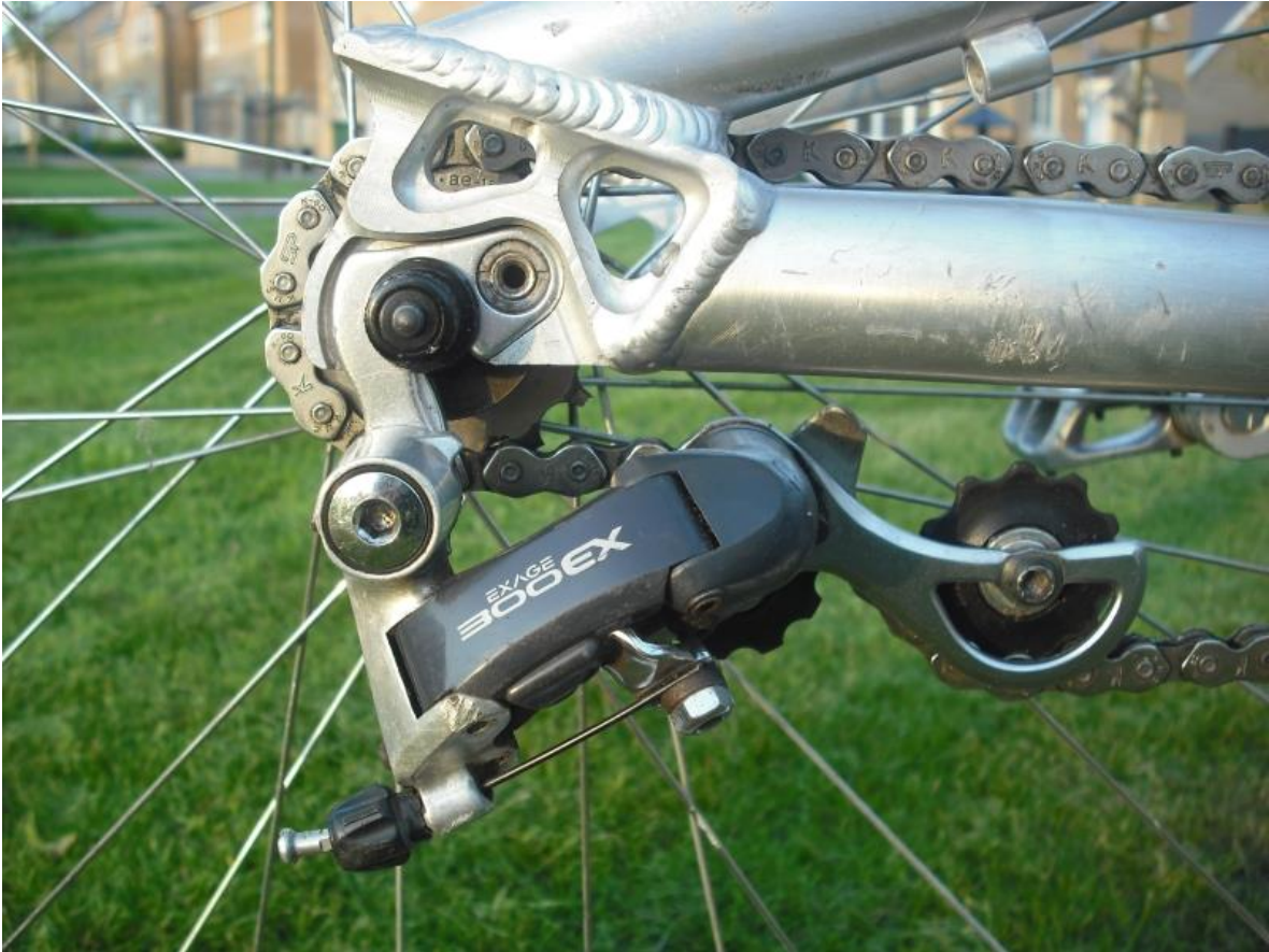
Figure 21: A typical single speed conversion. A short cage road mech acts as a tensioning device. It has been locked in gear with a cut down spoke and the cages have been spaced out to accommodate a wider, stronger chain.
