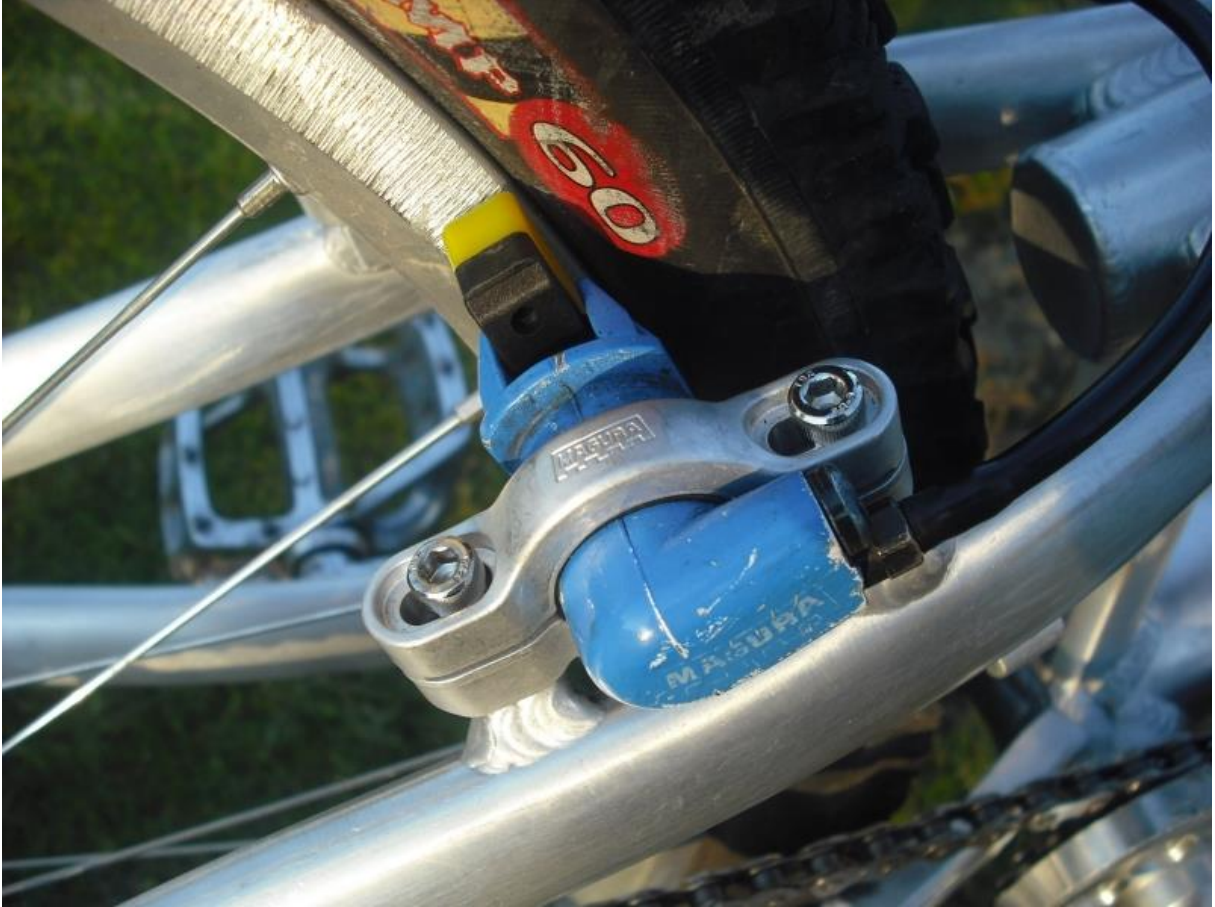
Figure 20: The hugely popular Magura HS33 rear hydraulic rim brake, four bolt mount, with home ground rim.
