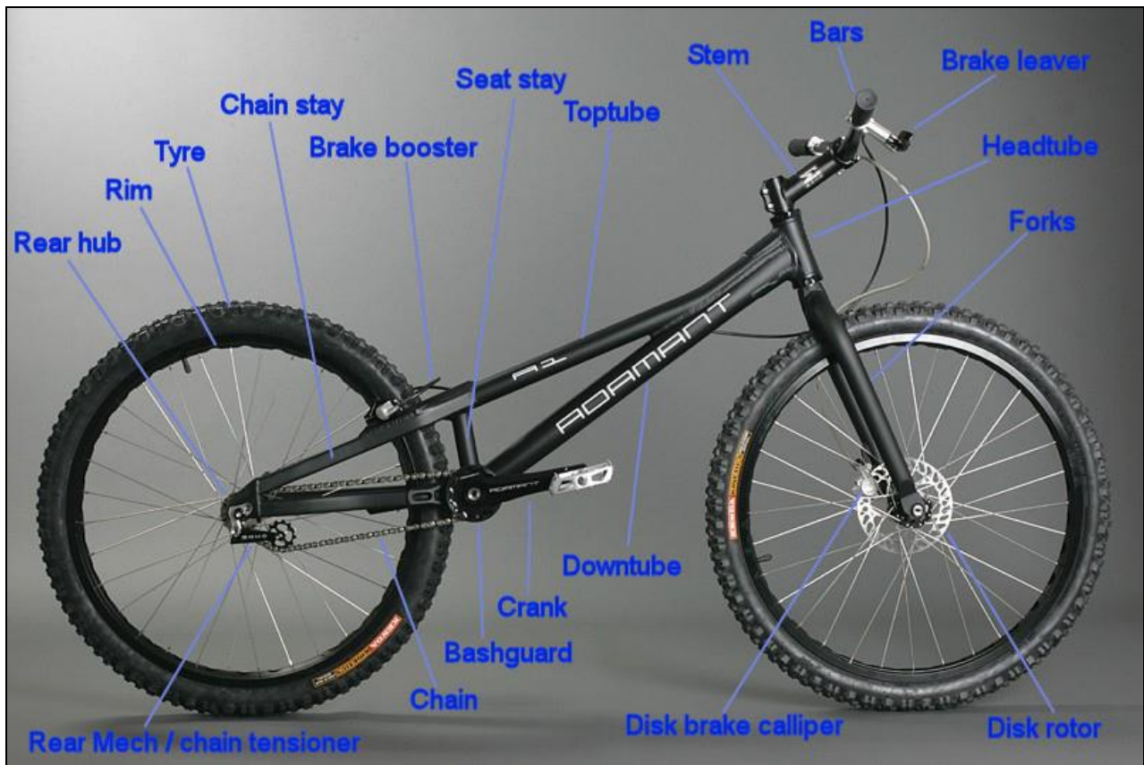
Figure 19: Anatomy of a stock trials bike. Labelling: author's, photo credit: Adamantbikes.com
