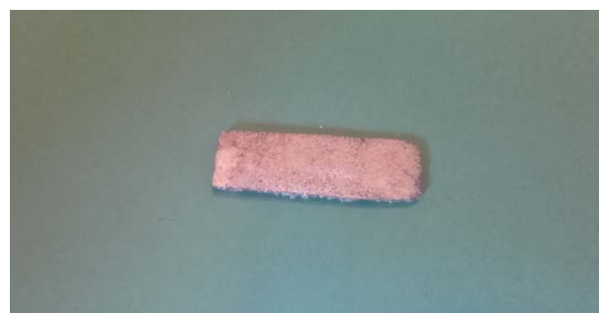
Fig. 3. SLM part of Cu-Ti-TiB 2 alloy from mechanically alloyed powder, obtained under process parameters of 20 Hz; 4 ms; 4 mJ.
