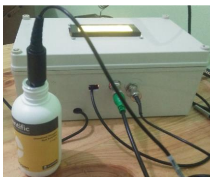
Gambar 8. Kalibrasi sensor DO
