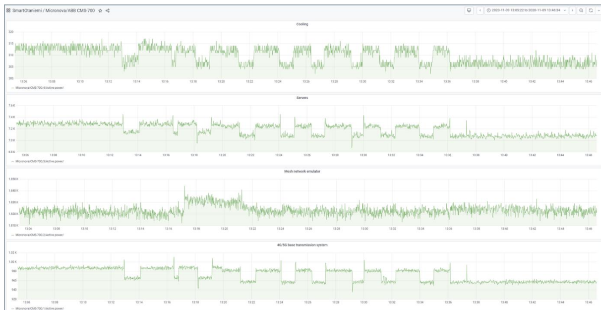
Figure 12. An example of an electric power real-time monitoring dashboard (case ABB CMS-700).
