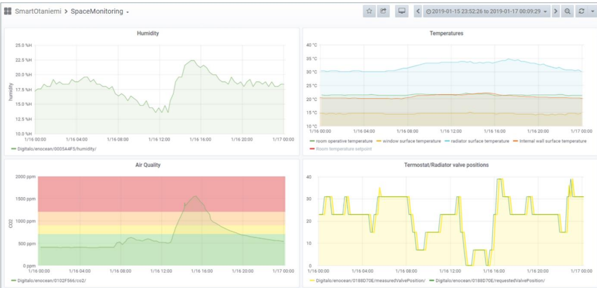
Figure 18. An example of the VTT research platform connected Grafana dashboard for monitoring space data (case Vuorimiehentie 3, Space A105, zoomed to one-day data).
