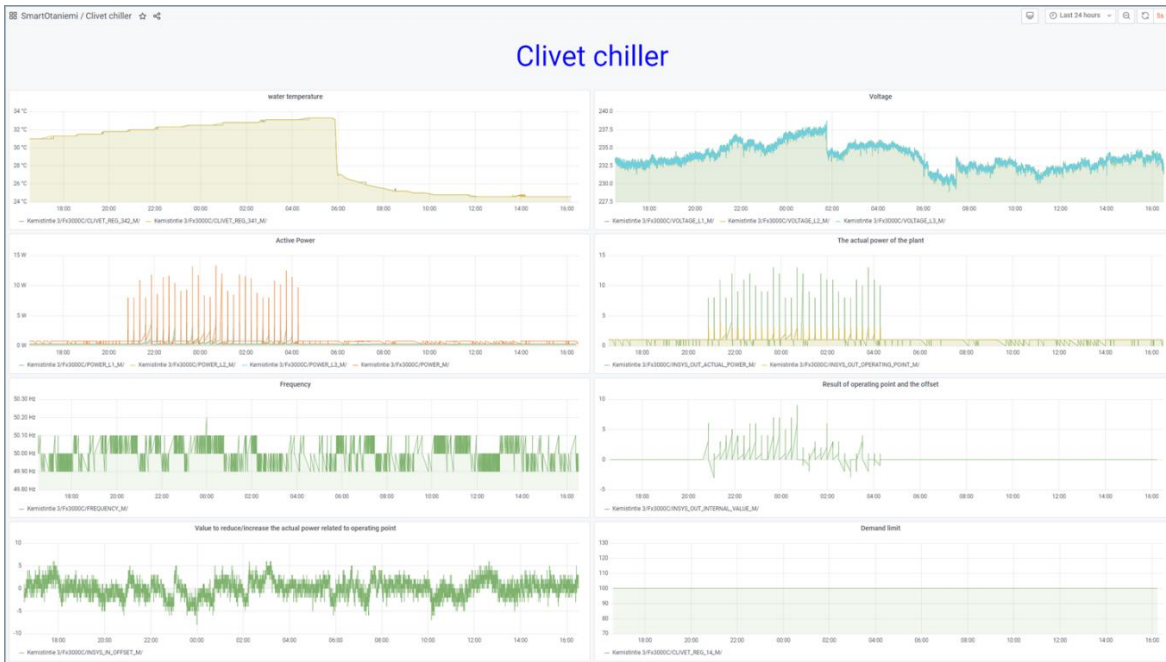
Figure 14. An example of a VTT research platform based chiller unit real-time monitoring dashboard (case Kemistintie 3 Clivet chiller unit via Fidelix FX-3000-C).
