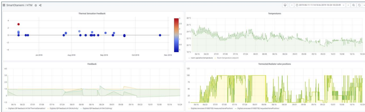
Figure 21. An example of a dashboard for digital twin based control of individual indoor thermal comfort (case studied human in Vuorimiehentie 3 space A104).
