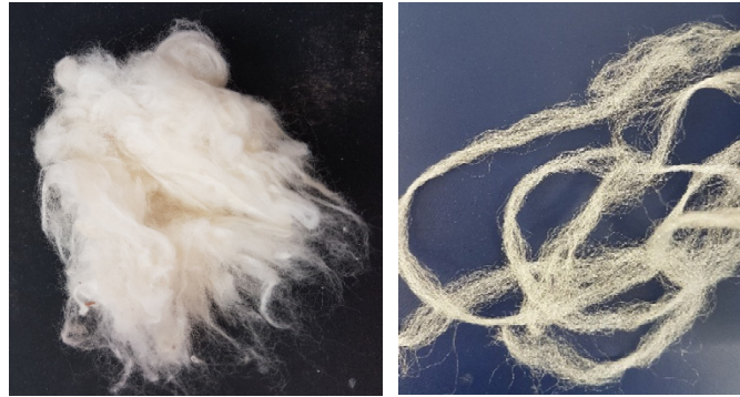
Figure 14 Virgin cotton staple fibres (vCOfref) and polyester filament fibres (vPESref) used for studying effect of cleaning process conditions
