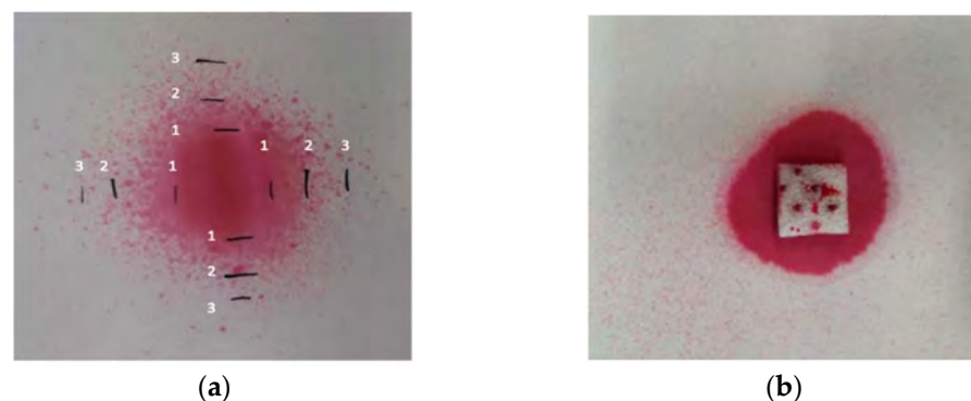
Figure 2. Distribution of an aqueous solution of Allura red AC observed when performing (a) 1 spray with different heights such as 2 cm (line 1), 3.3 cm (line 2), and 4.5 cm (line 3); (b) 3 sprays at previously optimized fixed height (4.7 cm).
