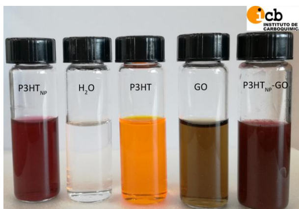
Figure 2.9. Dispersions of P3HT NPs (1st flask left) and P3HT NPs -GO (5th flask right). P3HT NPs were obtained by injection of P3HT dissolved in THF (flask in the middle) in water (2nd flasks from left). P3HT NPs -GO were obtained by injection of P3HT dissolved in THF in aqueous dispersion of GO (4th flasks from left).
