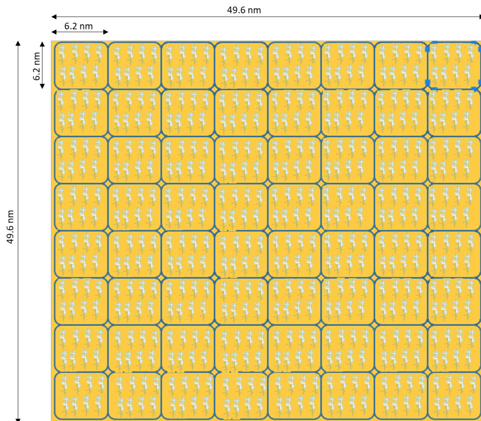
Figure S13. Illustration of binding sites per unit area of IOS-1 peptoid immunobiosensor
