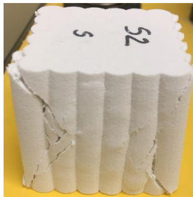
Figure 4.55 Shear 2 failure mode of Horn solid structures (Batch S).
