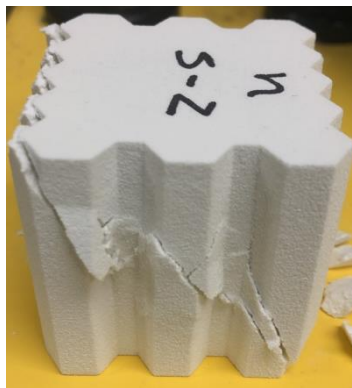
Figure 4.39 Shear 1 failure mode of Honeycomb solid parts (Batch N).
