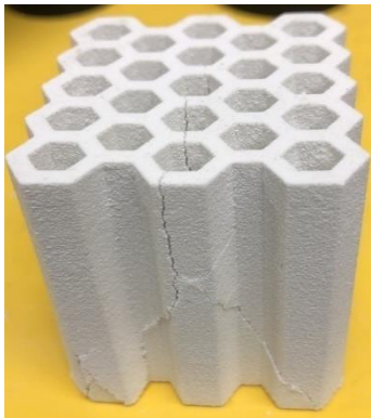
Figure 4.32 Shear 4 failure mode of Honeycomb cellular structures (Batch M).
