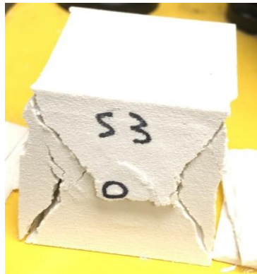
Figure 4.45 Shear 2 failure mode of Plant Stalk solid structure (Batch O).
