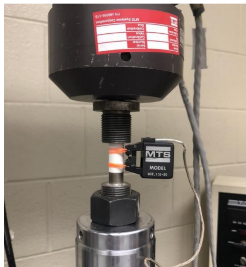
Figure 3.22 12x24 mm cylinder being tested under uniaxial compression with MTS loading device and extensometer.
