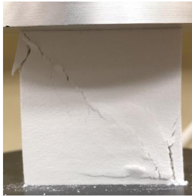
Figure 4.44 Shear 1 failure mode of Plant Stalk solid structure (Batch O).
