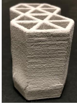
Figure 4.13 Buckling failure mode.
