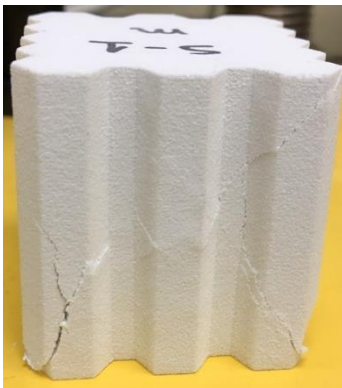
Figure 4.32 Shear 4 failure mode of Honeycomb cellular structures (Batch M).
