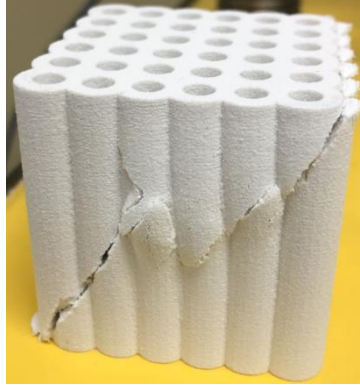
Figure 4.53 Shear 1 failure mode of Horn cellular structures (Batch S).
