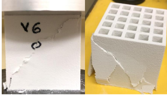
Figure 4.43 Shear 1 failure mode of Plant Stalk cellular structure (Batch O).
