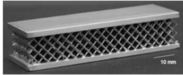
Figure 2.43 Diamond shape 304 stainless steel textile sandwich panel. (Wadley et. al., 2003)
