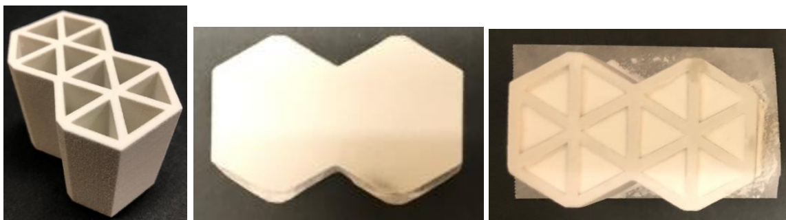
Figure 3.18 Toucan Beak IV 3D printed prototype with cellular, solid and infilled cellular structures, respectively.
