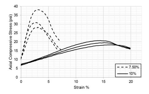
*Figure 26. Strain-stress relationship measure at 1 hour at 7.5% and 10% MC. Note: 1000 psi = 6.89 MPa.*
