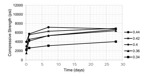
Figure 7. Compressive strength of wet specimens using 1.00 s/c. Note: 1000 psi = 6.89 MPa
