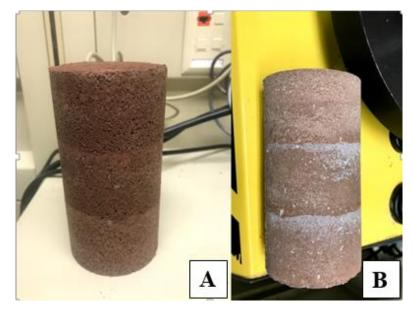
Figure 17. Comparison of soil-cement specimen using different binders tested at 7 days. (A) PC soil-cement specimen; (B) BCSA soil-cement specimen
