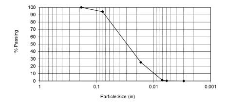
Figure 12. Gradation curve of the play sand. Note: 1 in =25.4 mm
