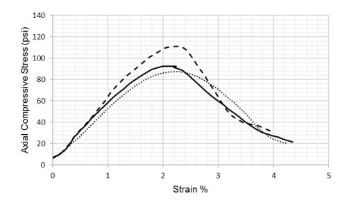
Figure 24. Strain-stress relationship measure at 1 hour using BCSA cement at 10% MC. Note: 1000 psi = 6.89 MPa
