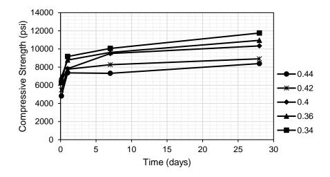
Figure 8. Compressive strength of dry specimens using 1.25 s/c. Note: 1000 psi = 6.89 MPa
