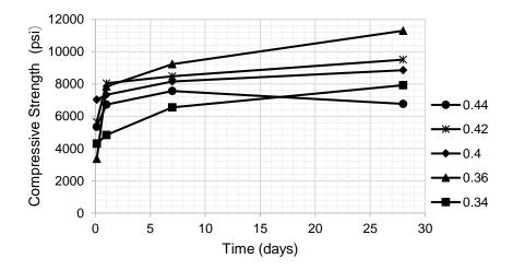
Figure 6. Compressive strength of dry specimens using 1.0 s/c. Note: 1000 psi = 6.89 MPa
