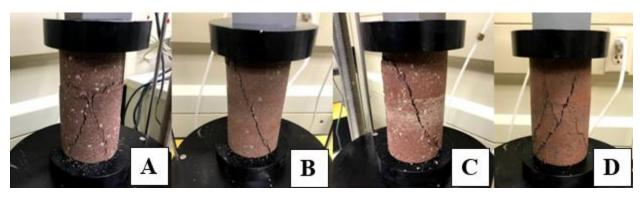
*Figure 20. Failure mechanism for soil cement specimens tested at 3 hours. (A) BCSA at 7.5% MC; (B) PC at 7.5% MC ;(C) BCSA at 10% MC; (D) PC at 10% MC.*
