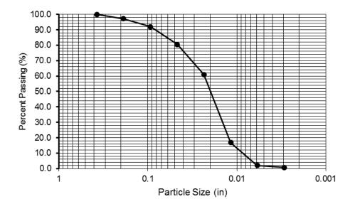
Figure 1. Sand Gradation Curve. Note: 1 in = 25.4 mm
