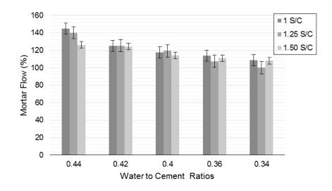
Figure 4. Mortar flow percent using different s/c and w/c.
