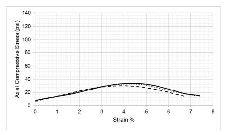
Figure 25. Strain-stress relationship measure at 1 hour using PC cement at 10% MC. Note: 1000 psi = 6.89 MPa.
