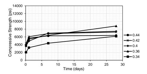
Figure 9. Compressive strength of wet specimens using 1.25 s/c. Note: 1000 psi = 6.89 MPa
