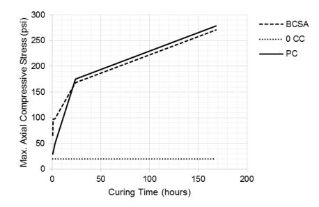
Figure 30. Maximum compressive strengths at 10 % MC. Note: 1000 psi = 6.89 MPa
