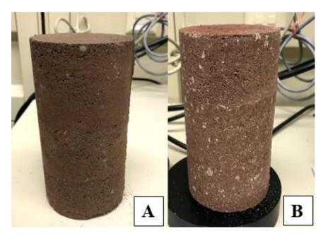
Figure 16. Comparison of soil-cement specimen using different binders tested at 1 hour. (A)PC soil-cement specimen; (B) BCSA soil-cement specimen
