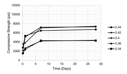
Figure 11. Compressive strength of wet specimens using 1.5 s/c. Note: 1000 psi = 6.89 MPa
