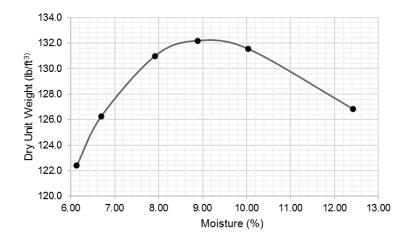
Figure 13. Compaction curve of the soil mixture. Note:  $1 \text{ kN/m}^3 = 6.3659 \text{ lb/ft}^3$
