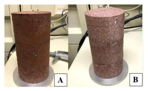
*Figure 19. Visual difference between specimens using both binders at 1 day. (A) PC specimen; (B) BCSA specimen.*
