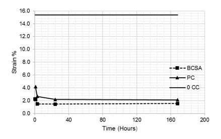
Figure 28. Strain at peak using 10% MC.
