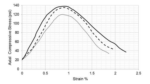
*Figure 22. Strain-stress relationship measure at 1 hour using BCSA cement at 7.5% MC. Note: 1000 psi = 6.89 MPa*
