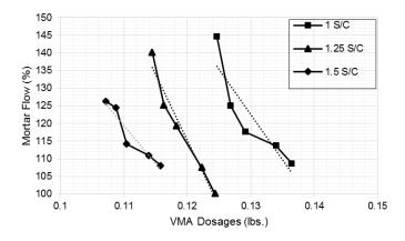
Figure 5. Relationship between the mortar flow and the VMA dosages. Note: 1kg = 2.2 lb; 1kg = 1000 g
