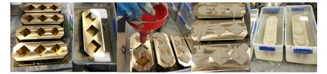
Figure 2. Fresh mortar specimen casting set-up.
