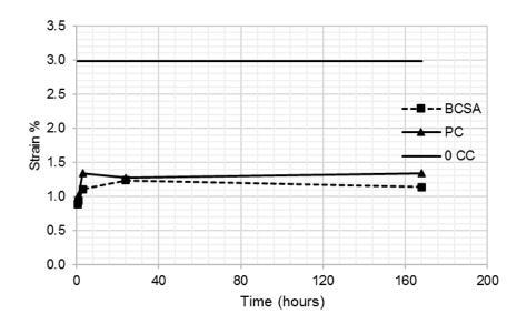
Figure 27. Strain at peak using 7.5% MC.
