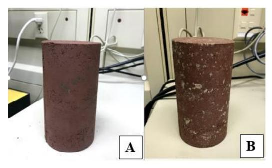
*Figure 18. Visual difference of samples using both binders at 10% MC. (A) PC specimen; (B) BCSA specimen.*
