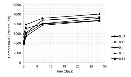
Figure 10. Compressive strength of dry specimens using 1.5 s/c. Note: 1000 psi = 6.89 MPa
