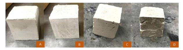
*Figure 3. Mortar cubes using different w/c and 1.25 s/c. (A) dry sample using a 0.42 w/c; (B) wet sample using a 0.42 w/c; (C) dry sample using a 0.36 w/c; (D) wet sample using a 0.36 w/c.*
