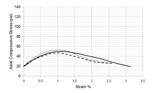
Figure 23. Strain-stress relationship measure at 1 hour using PC cement at 7.5% MC. Note: 1000 psi = 6.89 MPa
