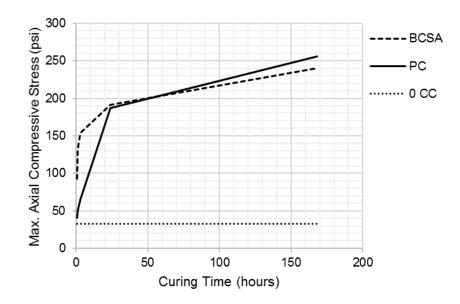
*Figure 29. Maximum compressive strengths at 7.5% MC. Note: 1000 psi = 6.89 MPa*
