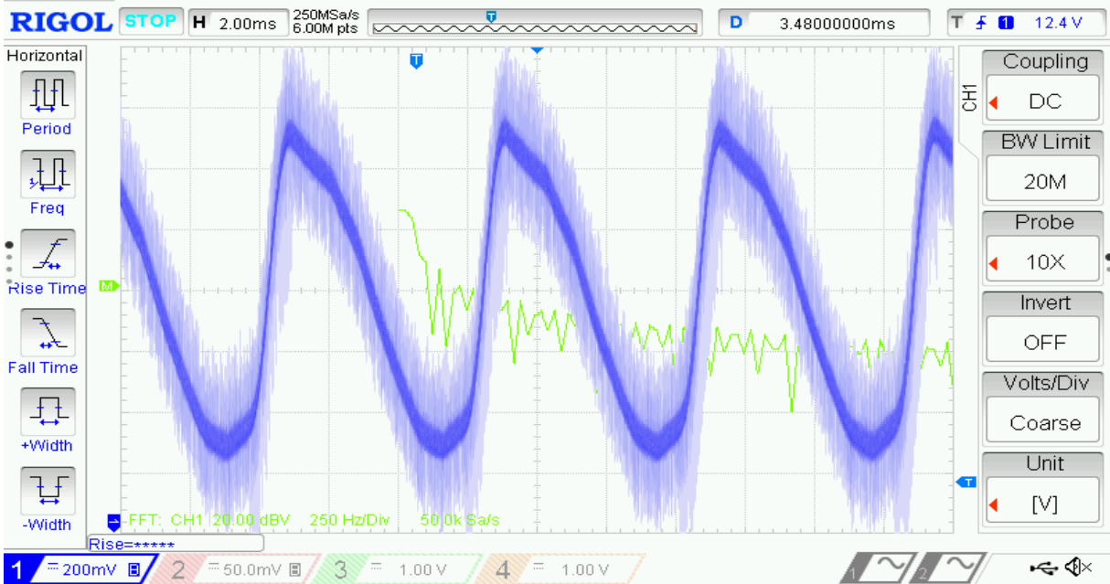
Figure 6.19: Experimental analyzing output voltage signal by FFT of the buck converter.
