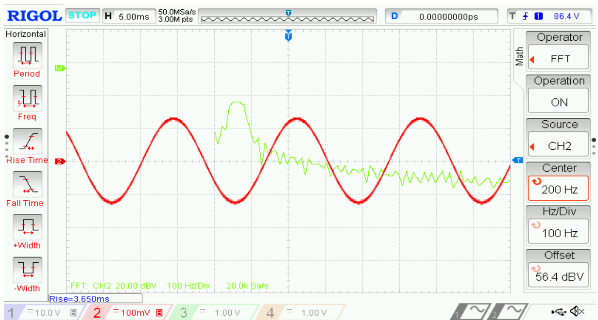
Figure 6.36: Experimental FFT analysis of control signal 60Hz the boost converter.
