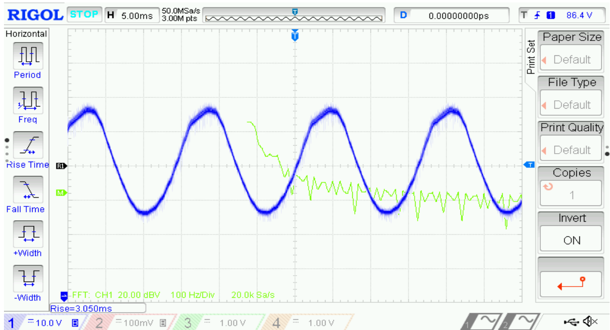
Figure 6.37: Experimental FFT analysis of output voltage boost converter.
