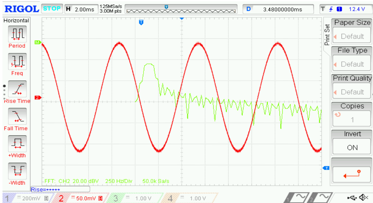
Figure 6.18: Experimental analyzing 10 KHz control signal by FFT of buck converter.
