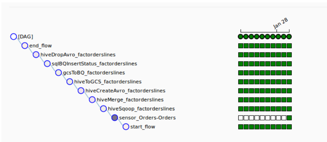
Figure 2.13: A oozie workflow DAG used at Farfetch
