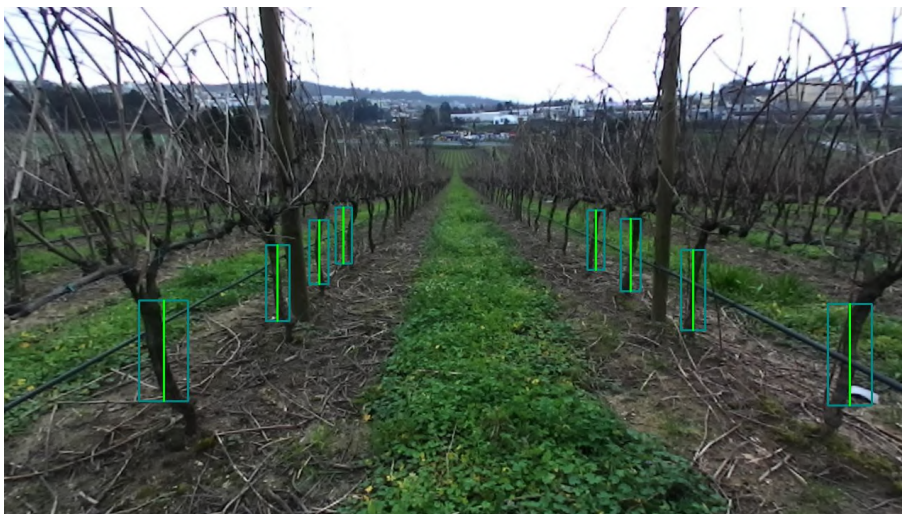
Figure 5.10: Real-time inference using Edge TPU for trunk detection.
