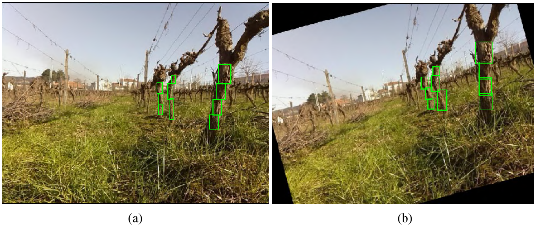
Figure 5.12: Result of an augmentation operation applying a -15 degree rotation on the (a) original image, resulting on the (b) augment image.
