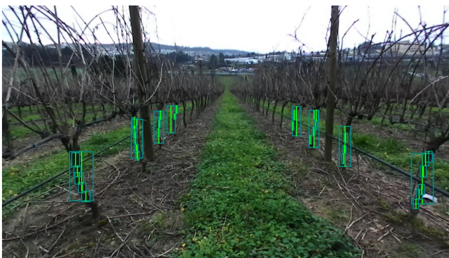
Figure 5.14: Real-time inference using Edge TPU for trunk detection and segmentation simultaneously.
