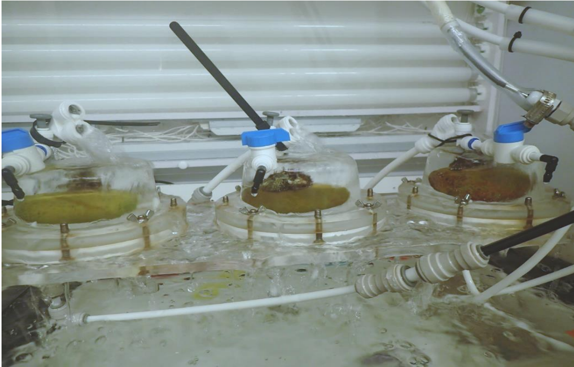
Figure 6: System to measure the oxygen consumption ( \mu\text{mol O}_2 \text{ g}^{-1} \text{ h}^{-1} ) with three chambers.
