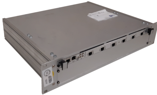
FIGURE 5.8: FlashCam FADC module used to digitalize all PMT signals.
