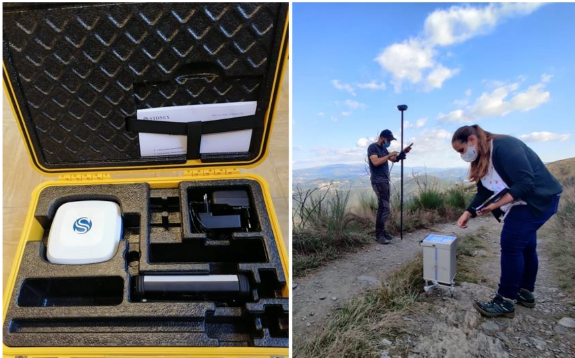
Figure 35 – On the left: differential GPS Stonex S850A in its case; On the right: Stonex S850A and gravimeter CG-5 Autograv being used on the field.
