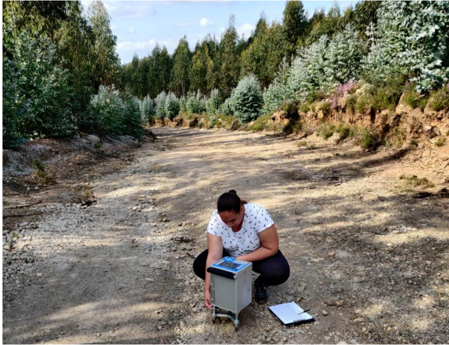
Figure 34 - Scintrex CG-5 Autograv gravimeter being levelled on the field to perform a reading.
