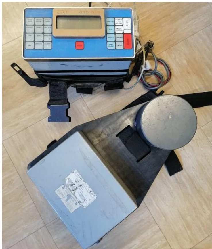
Figure 44 – EDA's OMNI PLUS equipment used in the electromagnetic survey. On the top of the image is the console and down is the antenna with the three-component sensor.
