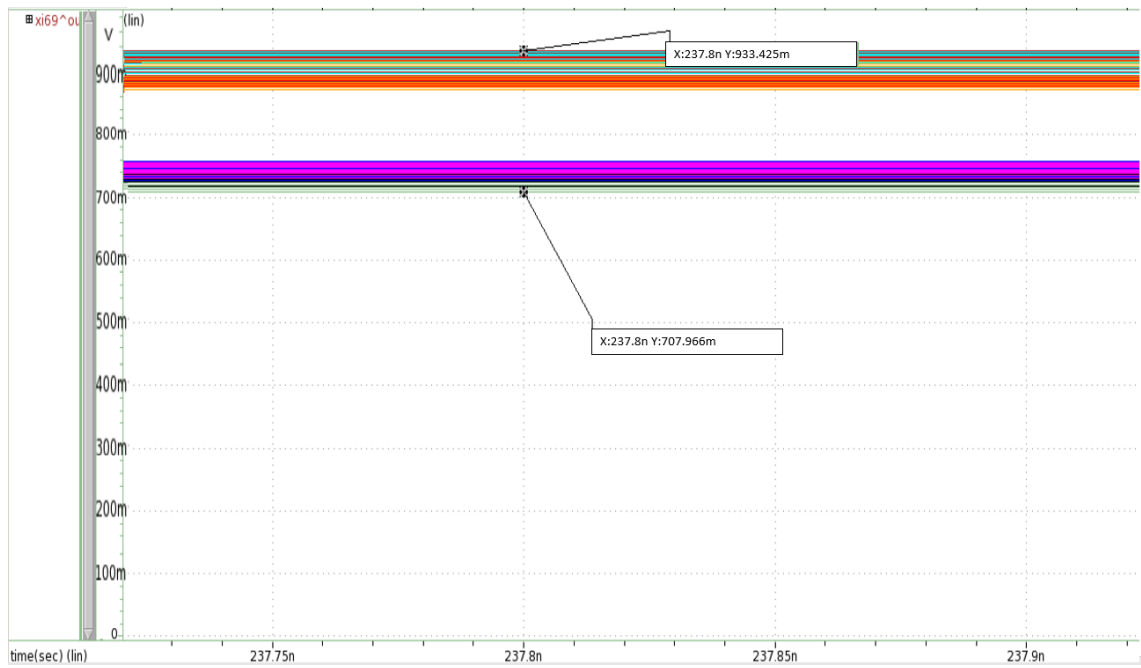
Figure B.14: Output of the FVC with 1.2 GHz input wave in the third range in PVT.
