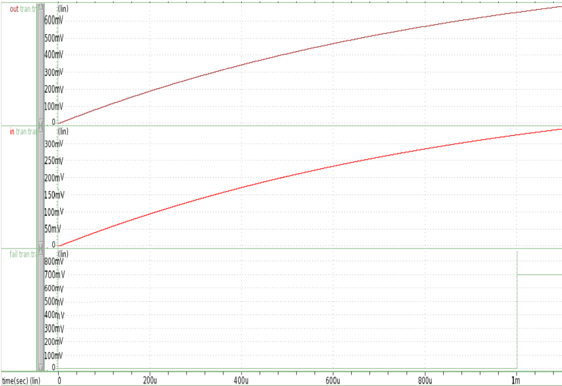
Figure 4.33: Voltage Regulator failing settling time test.
