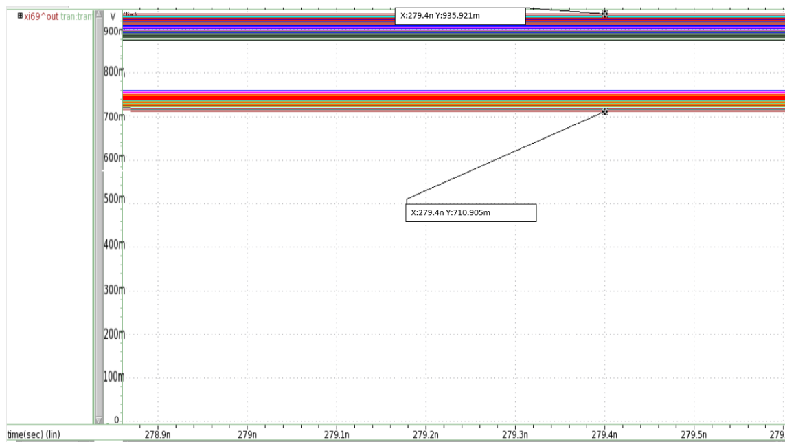
Figure B.16: Output of the FVC with 2.4 GHz input wave in the fourth range in PVT.
