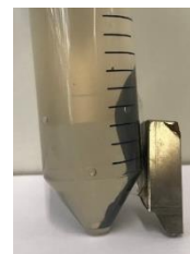
Figure 2.1. Magnetic separation of the MNPs by an external magnet.
