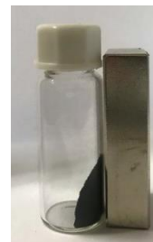
Figure 2.3. Magnetic separation of ZIF-DPC by an external magnet.
