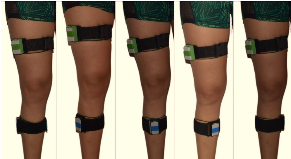
Figure 5.6 - Sensor placement: \phi_1 = -45^\circ and \phi_2 = -90^\circ, -45^\circ, 0^\circ, 45^\circ and 90^\circ (right to left).
