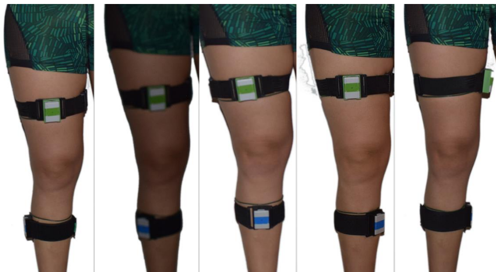
Figure 5.7 - Sensor placement: \phi_1 = 0^\circ and \phi_2 = -90^\circ, -45^\circ, 0^\circ, 45^\circ and 90^\circ (right to left).
