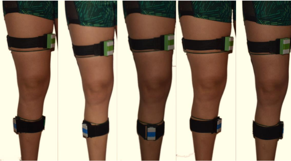
Figure 5.8 - Sensor placement: \phi_1 = 45^\circ and \phi_2 = -90^\circ, -45^\circ, 0^\circ, 45^\circ and 90^\circ (right to left).
