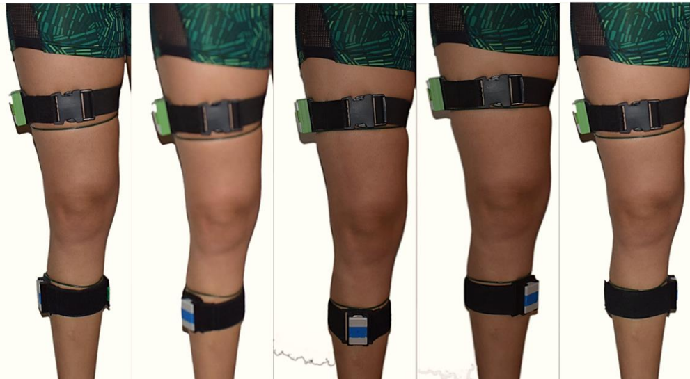
Figure 5.5 - Sensor placement: \phi_1 = -90^\circ and \phi_2 = -90^\circ, -45^\circ, 0^\circ, 45^\circ and 90^\circ (right to left).
