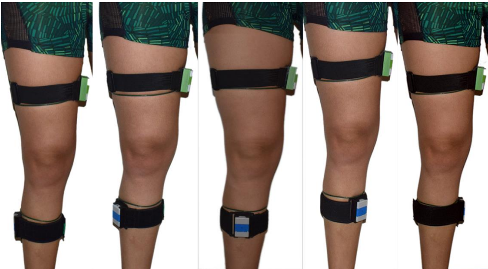
Figure 5.9 - Sensor placement: \phi_1 = 90^\circ and \phi_2 = -90^\circ, -45^\circ, 0^\circ, 45^\circ and 90^\circ (right to left).
