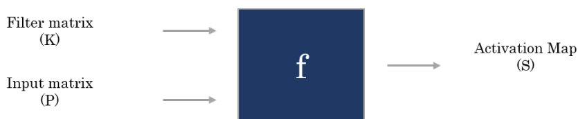
Figure 2.3: Simplistic visualisation of all the convolutions between a kernel K and the input matrix P , originating the activation map S
