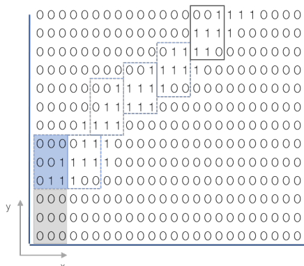
Figure 4.8: The algorithm "walks" inside a mask in 3x3 squares looking for lines identification.
