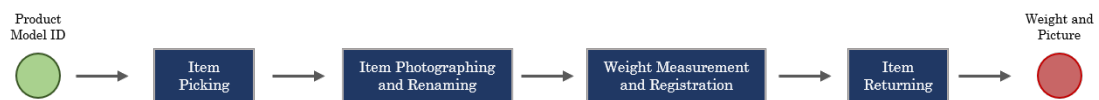
Figure 3.4: With this project, the manual item's width, depth and height measuring is replaced by a picture.
