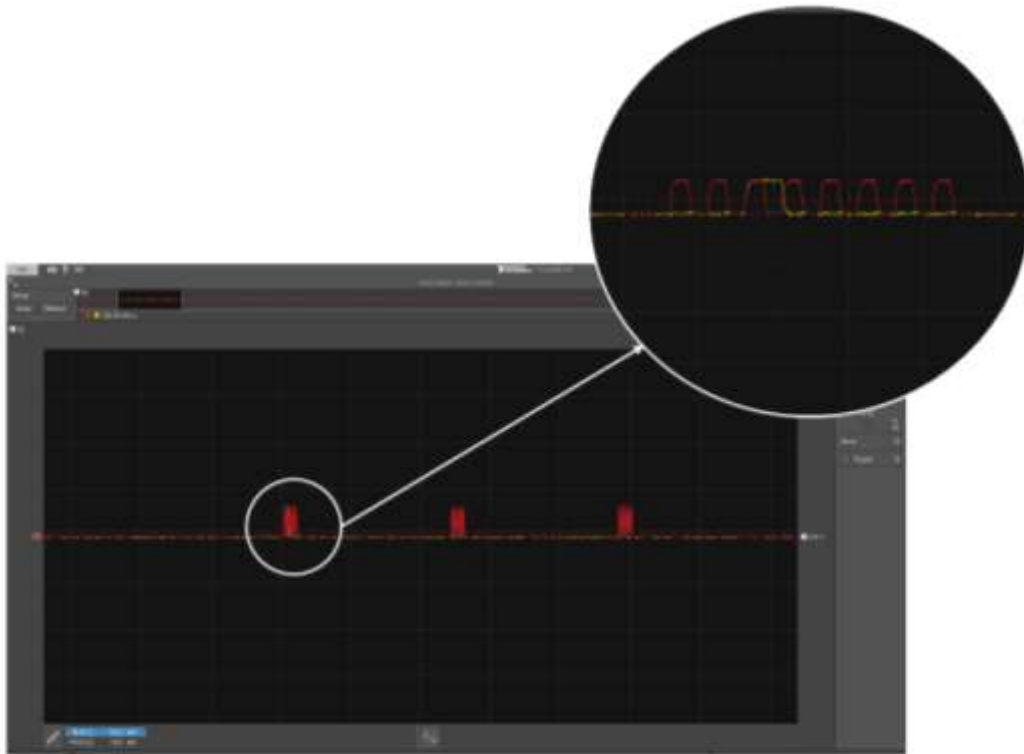
Figure 5.2 - Signal obtained in the implementation of the code to read the device ID. The red plot represents the serial clock, and yellow represents the master out (First byte 0b00100000; second byte 0b00000000; third byte 0b00000000).
