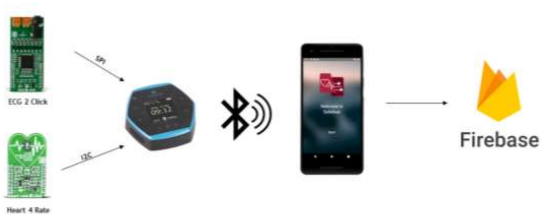
Figure 4.1 - Final system architecture scheme.
