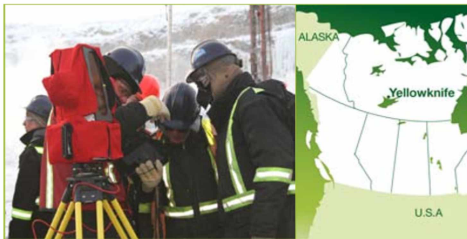
Figure 3. 3 I-Site 4400 scanner with protective jacket to keep out the cold (Maptek I-Site, 2008)
