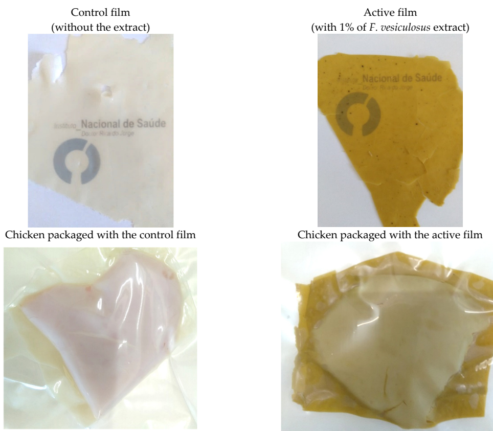
Figure 1. Control film (left) and active film with 1% of F. vesiculosus extract (right).
