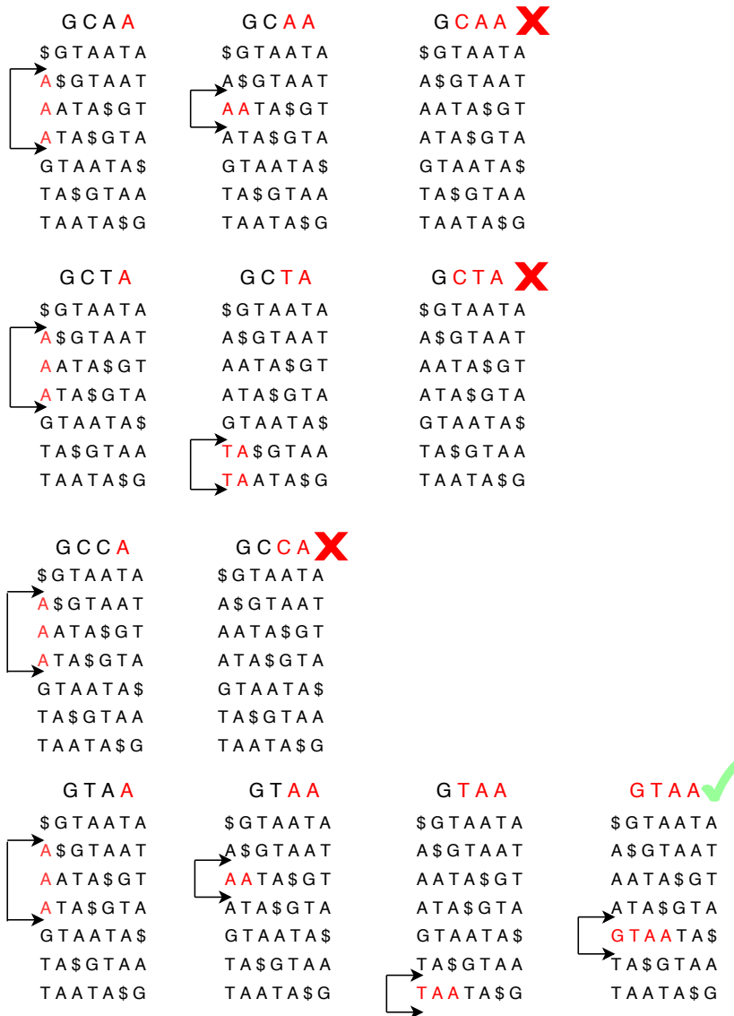
Figure 2.3: Bowtie: Inexact matching diagram
