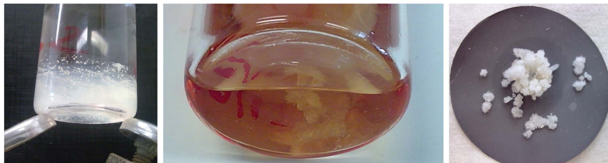
Fig. 1 Initial stages of crystal formation in the alginate gel (left). Crystal growth (middle). Isolated single crystals (right).
