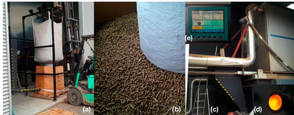
Figure 4. Combustion test of the pellets in an industrial thermal oil boiler. (a) The discharge of a pellet big bag into the boiler feed system; (b) the detail of the pellet discharge; (c) the boiler where the test was conducted; (d) the detail of the “eye” of the furnace in full combustion; and (e) the boiler control unit and the operating parameters.
