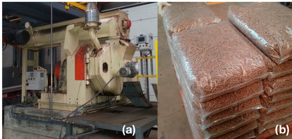
Figure 3. The production of pellets in industrial scale test. (a) The equipment used in the test: a LaMeccanica pelletizer with a production of 1200 kg/h; and (b) the produced pellets bagged and ready to be consumed in domestic equipment.
